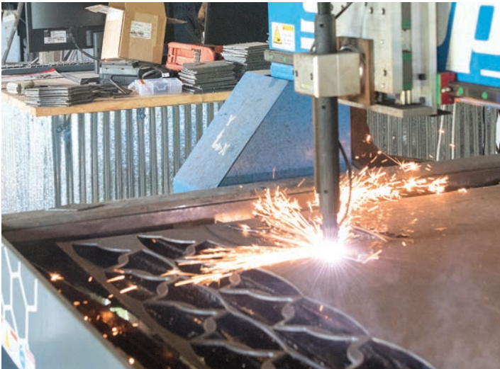
TOP LEFT: Will uses a wire wheel to clean up the weld on a hand-forged trowel. BOTTOM LEFT: To speed production, Will has embraced modern technologies such as this plasma cutter, which allows him to cut out tool shapes quickly and more efficiently. RIGHT: Adding a twisting to a tool shank ensures that when the handle is installed, it stays put without glue or epoxy. Will says it's an old-school trick that railroad tie hackers once used to keep their spikes from pulling out of the ties as they floated down Ozark streams.
